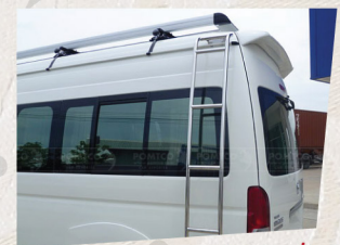
Roof rack Side ladder
